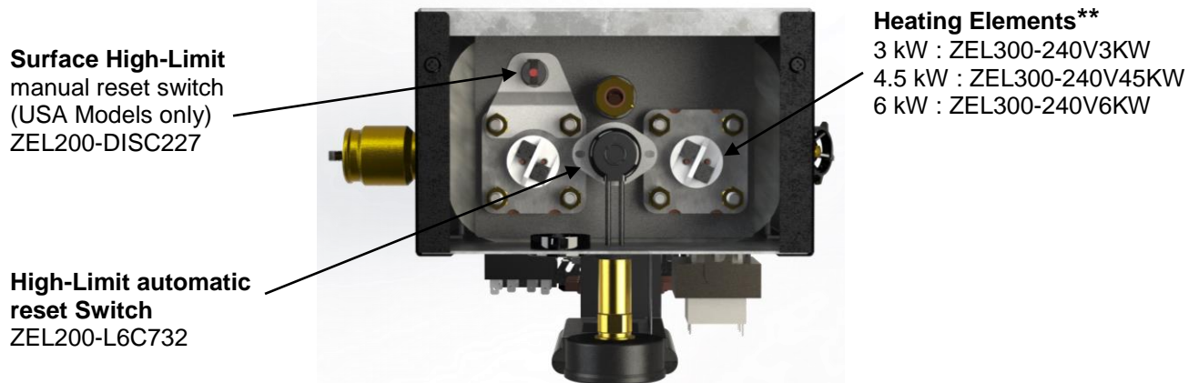
Figure 12 : Replacement Parts (Top view)
