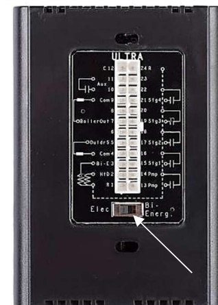
Figure 9: Back of the Controller
