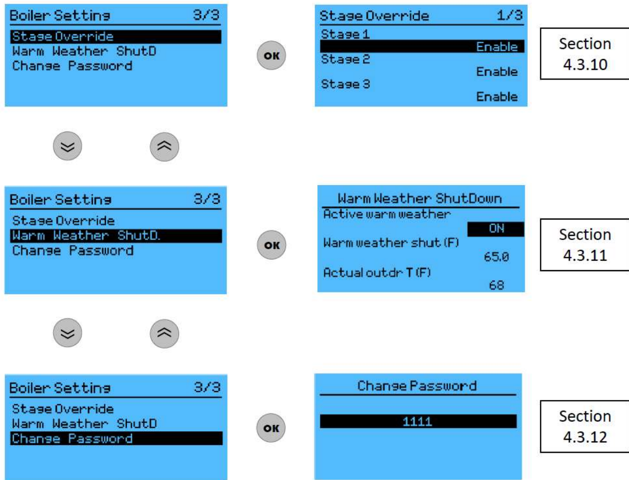
Figure 16 : Navigation in boiler setting menu (3/3)
