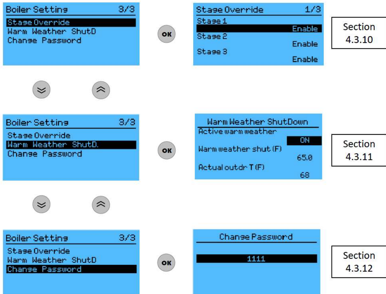
Figure 16 : Navigation in boiler setting menu (3/3)
