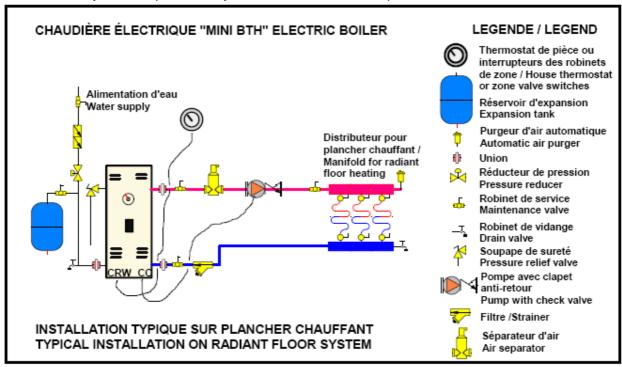
Figure 3: Typical piping lay-out
