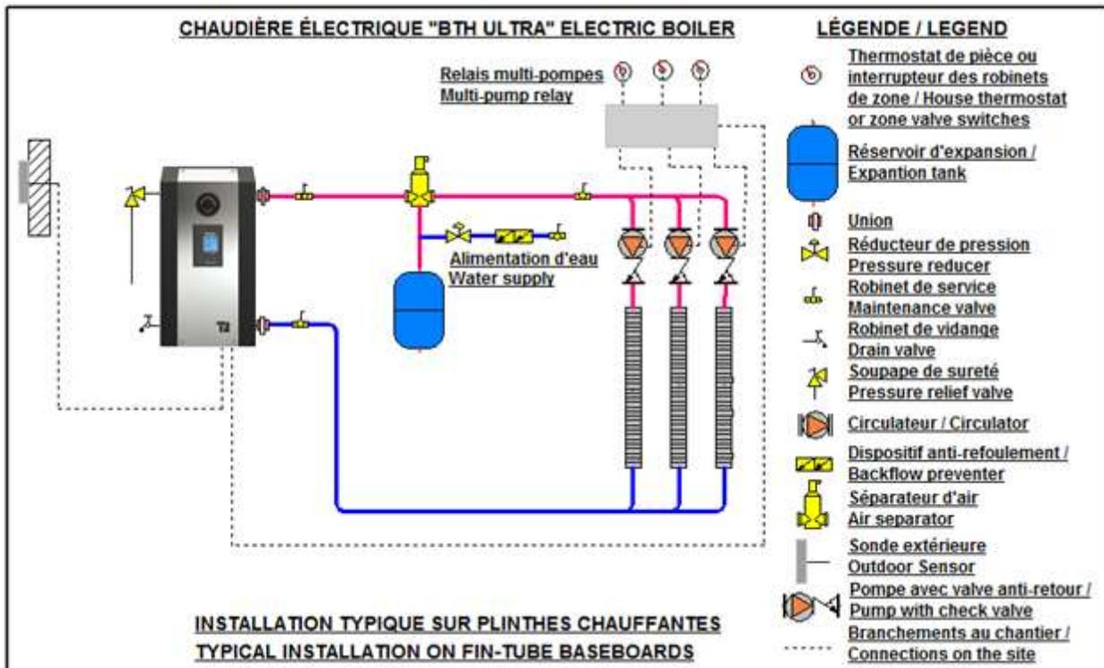
Figure 6 : Installation multi-pompes
