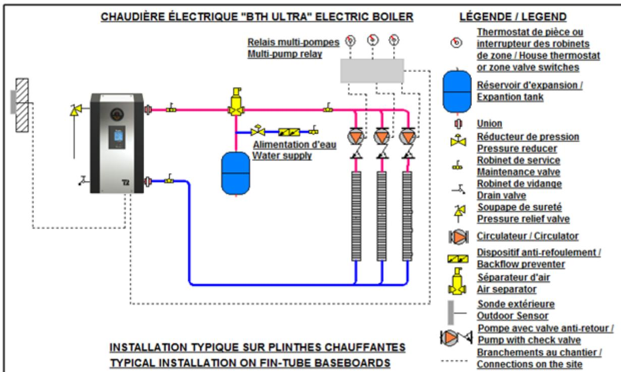
Figure 6 : Installation multi-pompes
